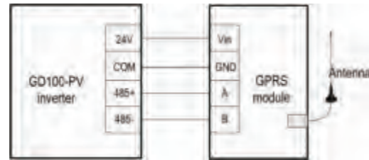
Diagram of connecting the GPRS module to the inverter
